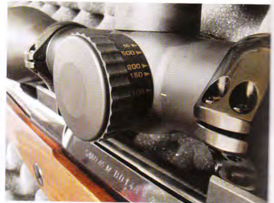
Vixen Parallax Adjustment Knob
