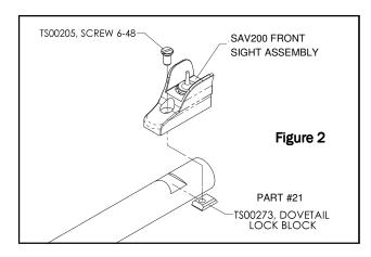
6. Slide or tap the Dovetail Lock Block into the dovetail slot until the tapped hole is centered on the barrel. (Fig. 2)
